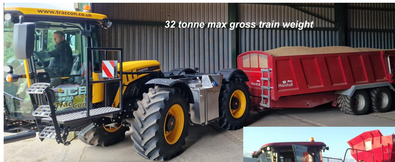
Twin line air brakes enable towing at up to 60 kph
